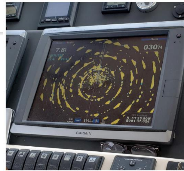
FIGURE 1.3 Photograph of the display of a shipboard radar operated in a U.K. wind farm. SOURCE: Sea-freeze, Ltd., included in public comments submitted to the 2019 U.S. Coast Guard Port Access Route Study: The Areas Offshore of Massachusetts and Rhode Island (USCG-2019-0131-0026).
